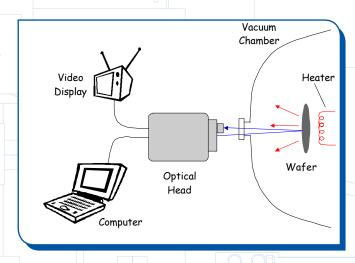
The schematic diagram above shows the layout of the In-Situ 4000 system. The integrated optical head contains the reflectometer illumination source, computer communications interface, and a video camera for ease of aiming and alignment with the substrate.
