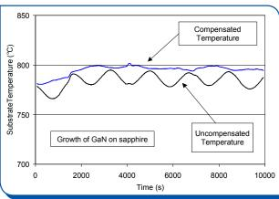
The figure above shows the temperature error which can occur when depositing multilayer thin films. The graph shows the measured substrate temperature during the MBE growth of GaN on sapphire. The lower curve shows the temperature as measured using traditional pyrometry while the upper curve shows the temperature after compensation by the reflectometry system.
